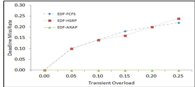
Figure 6: Hard Real-Time task miss rate (RTSIM)
