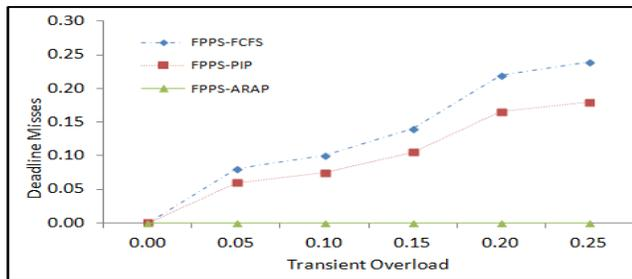
Figure 8: Hard Real-Time task miss rate (vxWorks)
